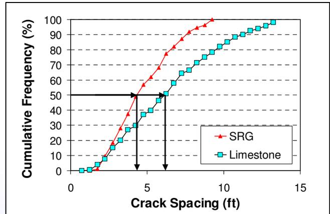
From these results, it can be concluded that CRCP will have better long-term performance provided the concrete used in its construction has a low CTE. In this case study, changing the aggregate in the concrete from one with a high CTE to one with a low CTE resulted in a larger average crack spacing. This translates to less distress in the long-term.
