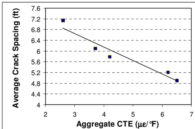
For aggregate with a low CTE, the crack spacing is high (6.8 ft), which translates to a reduced number of punchouts in the long-term.
