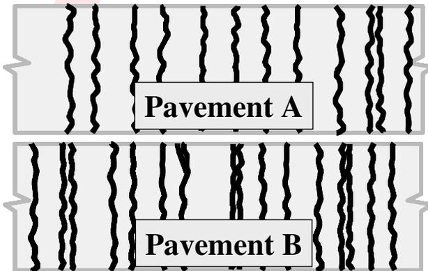
Further investigating the reasons behind this performance difference, Joe studies the construction documents to see if there is a difference in materials used or construction procedures followed when building Pavements A and B. The only difference he can find is that limestone aggregate was used in
