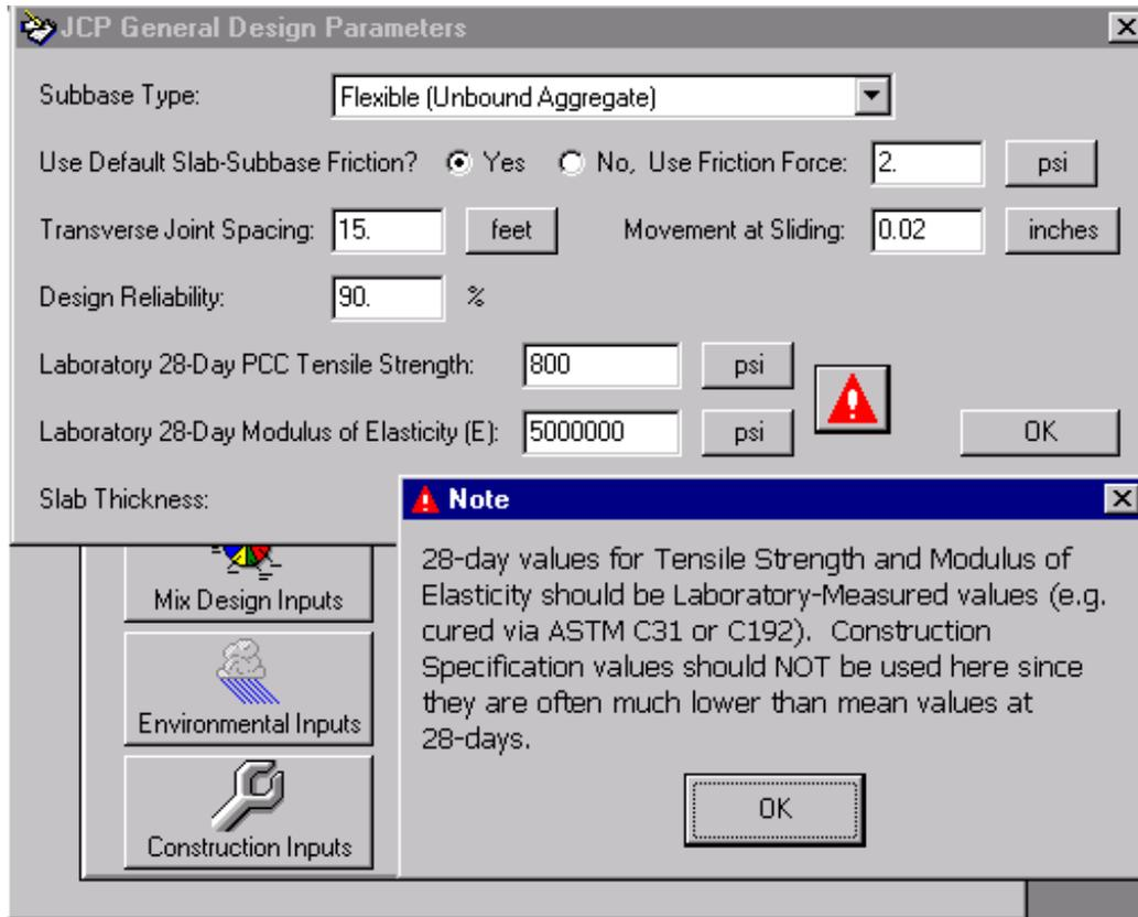
Figure 9. HIPERPAV Version 2.4 JCP general design parameters note.
