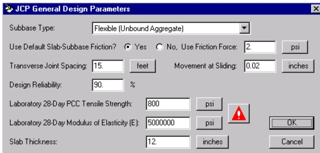
Figure 7. HIPERPAV Version 2.4 JCP general design parameters.
