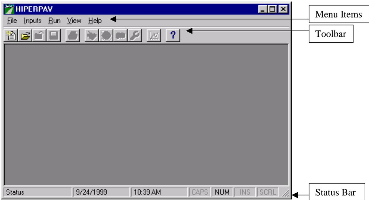
Figure 2. HIPERPAV Version 2.4 main menu components.
