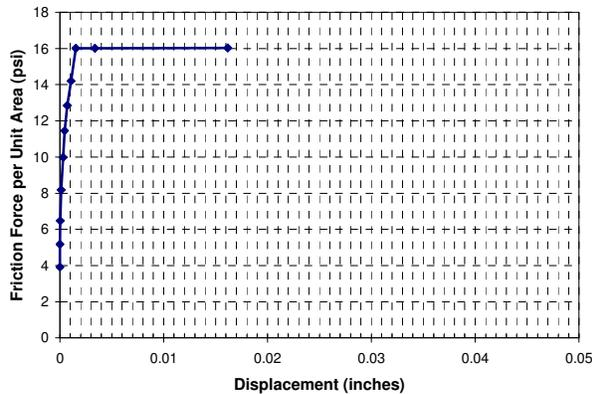
Figure 2. Typical Friction Curve for rough HMA base
