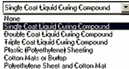
USER NOTE: Curing method may be a modification if HIPERPAV runs show that early age cracking of the pavement will happen.
