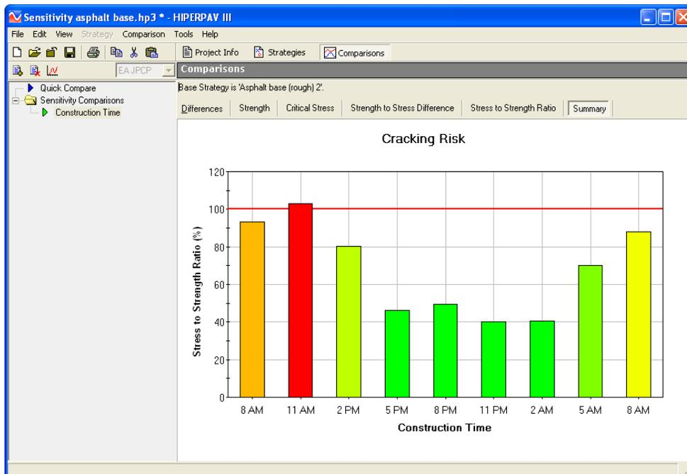
Figure 5 Construction Time Sensitivity
