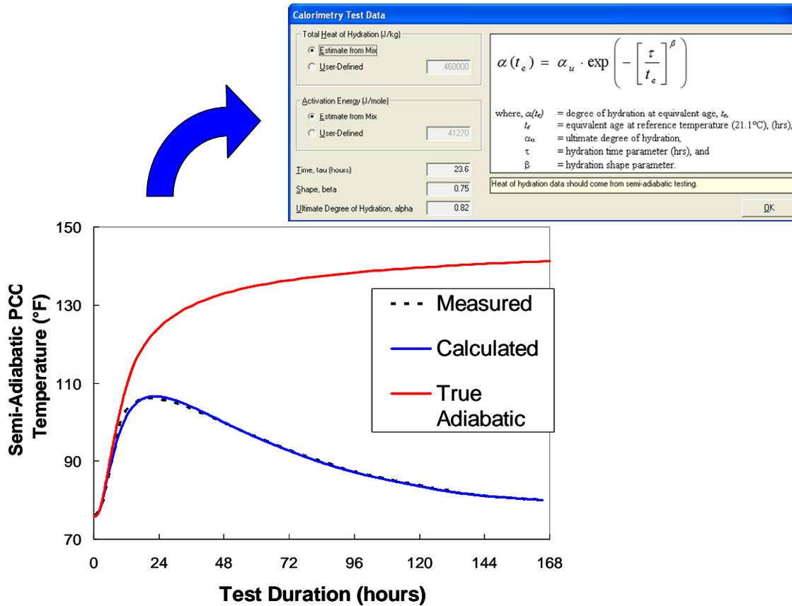
Figure 7 Heat Evolution Characterization from Semi-Adiabatic Calorimetry
