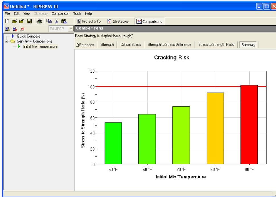
Figure 4 Mixture Temperature Sensitivity
