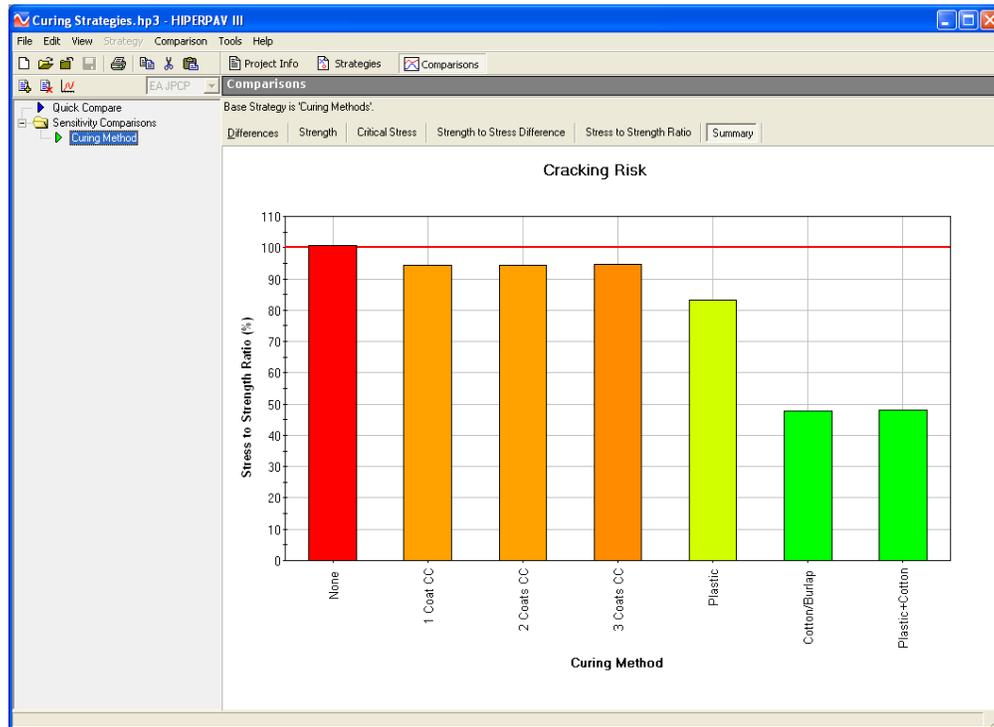
Figure 6 Effect of Curing Methods on Cracking Risk
