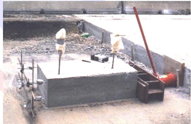
Figure 1. Setup for push-off test.
