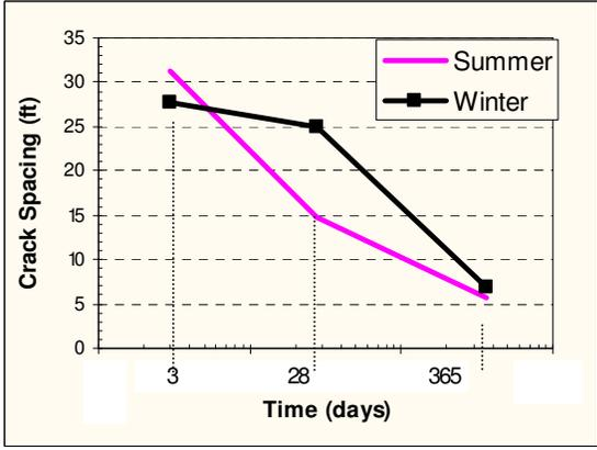
For both the summer and winter placements, increasing the temperature differential in the pavement (increasing  $\Delta T$ ) causes the crack spacing to decrease. As  $\Delta T$  increases, the slab is subjected to a larger temperature change as shown in the figure below. This means that more cracks are likely to form, since cracking in concrete pavements is highly influenced by temperature variations.
