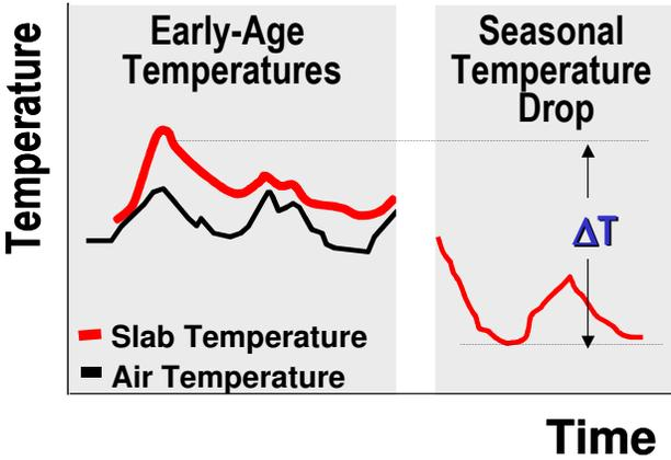
HIPERPAV takes into account the thermal processes due to the concrete’s heat of hydration, the curing temperature, the daily minimum temperatures and the annual minimum temperature when predicting crack formation. A cumulative frequency plot of crack spacing at one year for the summer and winter placements (with  $\Delta T = 60^\circ\text{F}$  and  $22^\circ\text{F}$ , respectively) is shown below. The trend at one year is consistent -- the CRCP placed in the summer has closer cracks.
